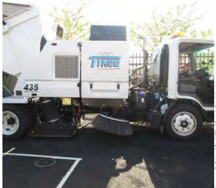
A regenerative air sweeper cleaning permeable pavement.
