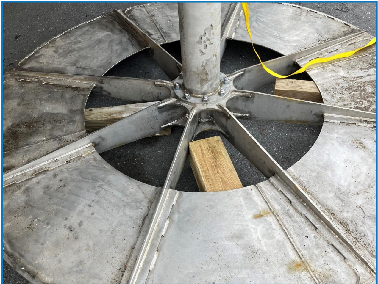
New Linear Motion Mixer Blade for installation on Primary Digester No. 2.
