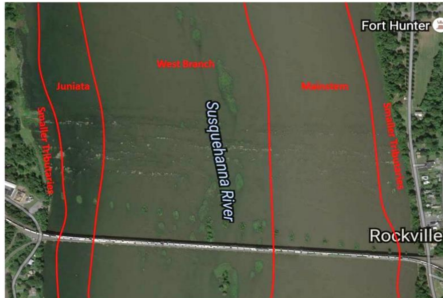
Figure 4. Approximate Extent of Lateral Mixing in the Susquehanna River at Rockville (PADEP, 2016)
