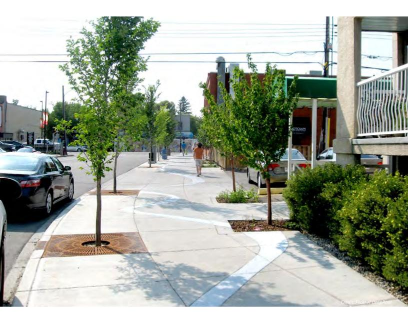
The size of stormwater tree trenches is flexible. Depending on its size, this type of system has the potential to manage a large volume of stormwater with a relatively small surface footprint. Given the large underground component of this system, maintenance is more extensive than what is required for a stormwater tree. Maintenance requirements include removing debris, cleaning inlets and overflow, trimming tree limbs, and occasional surveys to ensure that the trees remain healthy.
