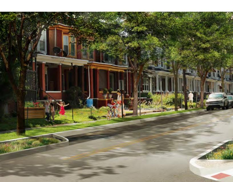
a more welcoming pedestrian environment. A small rain garden, flow-through planter, and rain barrel manage stormwater runoff from roofs on the eastern side of the street.
